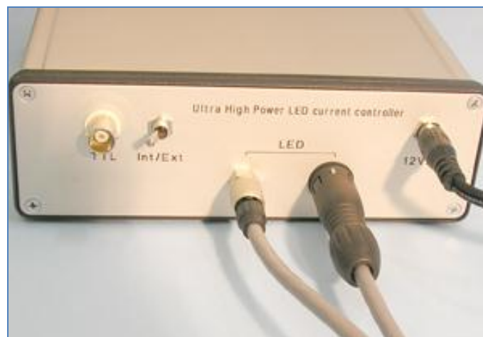
Figure 5: Cable connections on the rear panel of the UHP-LED-Current-Controller
