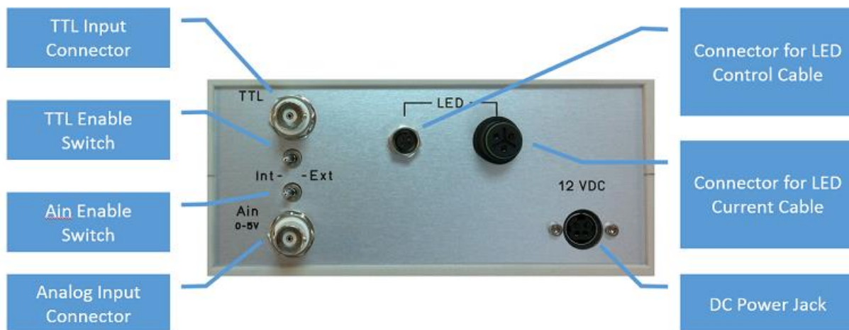
Figure 2: Rear panel of UHP-T-LED Current Controller
