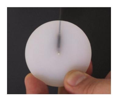
Place the puck on the polishing paper, and start polishing in figure-8 patterns or small circles.
