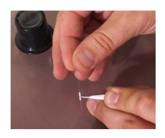
Push fiber through to desired length, measuring with caliper to get exact length.
