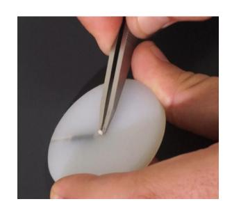
Tip: place the puck on several layers of tissue paper when inserting cannula
