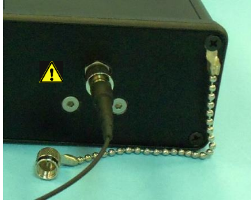
Fig. 6: Optical Fiber connected to the SMA port.
