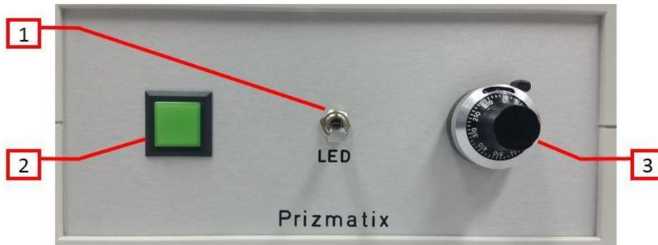
**Figure 1:** Front panel of UHPTLCC Current Controller: (1) LED on/off toggle switch, (2) Main power switch, (3) Power adjustment dial (10-turn potentiometer).
