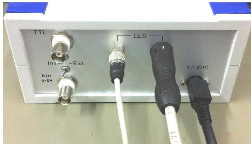
**Figure 5:** Cable connections on the back panel of the UHPTLCC LED current controller
