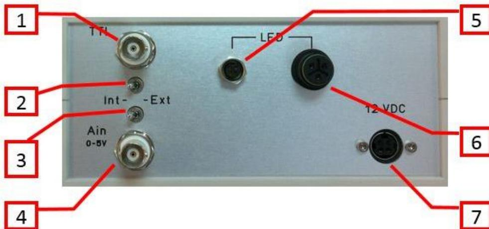
**Figure 2:** UHPTLCC LED Current Controller - back panel: (1) TTL input connector, (2) TTL-enable toggle switch, (3) Analog input (Ain)-enable toggle switch, (4) Analog input (Ain) connector, (5) LED control cable connector, (6) LED current cable connector, (7) DC power jack.
