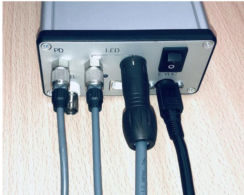
Figure 5a: Cable connections on the back panel of the UHPTLCC-02-STBL current controller. Remark: PD-LT Photosensor Cable has 5 pin metal connector; LED Control Cable has 4 pin metal connector.
