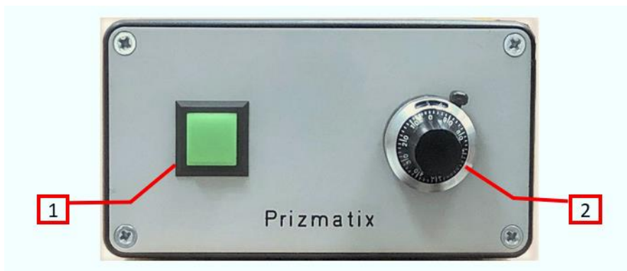
Figure 1: Front panel of UHPTLCC-02-USB Current Controller: (1) LED light On/Off switch with internal LED indicator, (2) Power adjustment dial (10-turn potentiometer).
