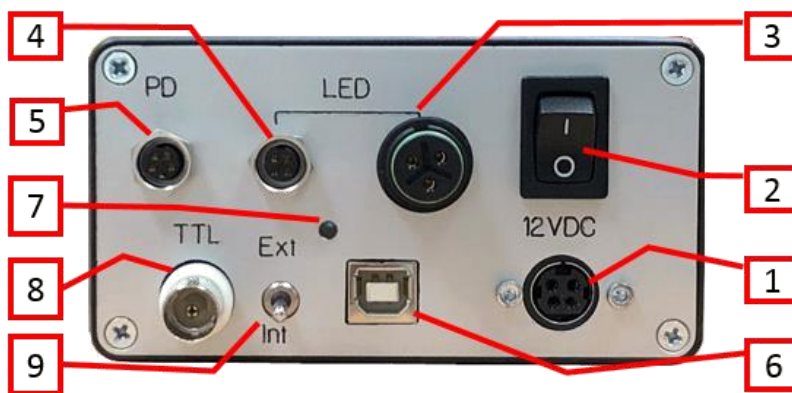
Figure 2: UHPTLCC-02-USB LED Current Controller - back panel: (1) 12V DC power jack, (2) Power On/Off switch, (3) LED current cable connector (3 contacts), (4) LED control cable connector (4 contacts), (5) Photosensor connector (5 contacts), (6) USB connector, (7) Indicator LED, (8) TTL input connector, (9) TTL-enable toggle switch.
