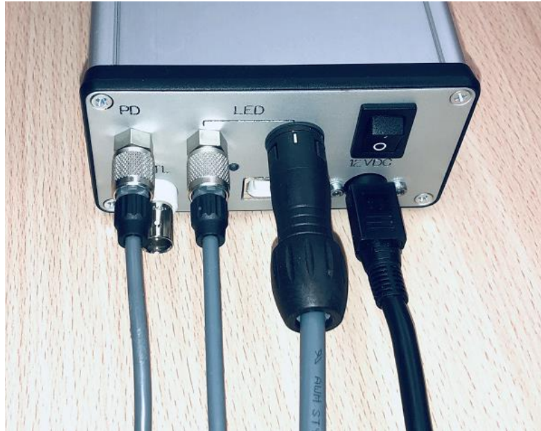
Figure 5a: Cable connections on the back panel of the UHPTLCC-02-USB current controller. Remark: PD-LT Photosensor Cable has 5 pin metal connector; LED Control Cable has 4 pin metal connector.
