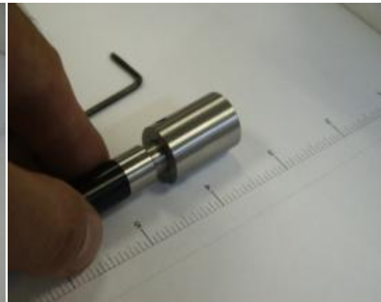
Collimator is set a bit forward
