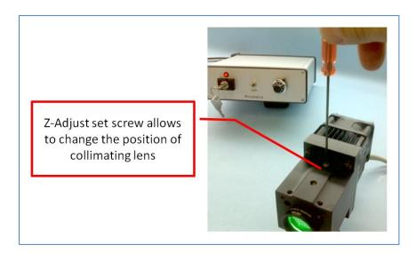
The correctly collimated beam shall be checked at a far field (few meters from the LED head).
