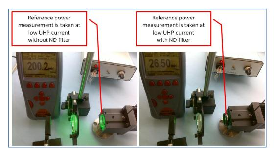
f) Increase the power dial to maximum current and take the attenuated power measurement.
