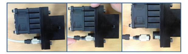
5) Use tweezers to press the small stoppers on the back of the connector while pulling the metal collar out. Remove the metal collar and use tweezers to open the two plastic shells of the connector body:
