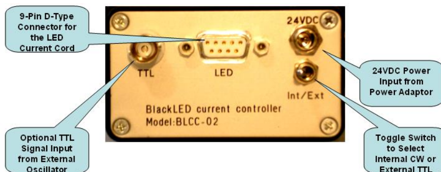
Fig 2: BLCC-2 Current Controller Back Panel
