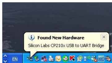
After few moments the driver will automatically recognize the device. At this stage the installation has been completed.
