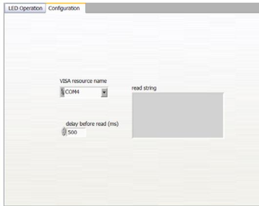
There is no need to change other settings. After selection of appropriate COM port close the software and re-open it again, check that the COM port is correct.
