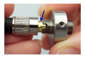
Push in fiber to the end, then pull the collar down towards the Rotary Joint. Holding the stator still, turn the collar to screw on fiber connector:
