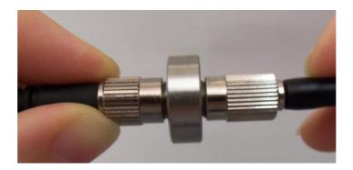
Now the fibers are connected to the Rotary Joint and ready to be attached to your light source. To detach fibers follow the same procedure in reverse.
