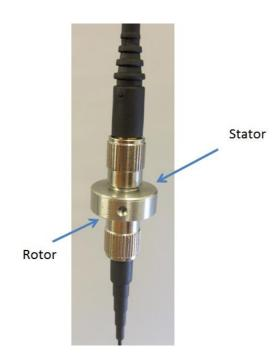
Pull back the collar around the fiber's connector to reveal a small key (the rounded protrusion), which matches with the small notch on the stator of the Rotary Joint:
